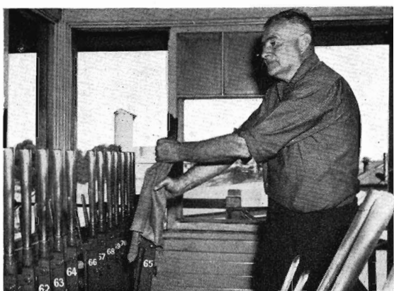
Signalman W. S. Aicken swings on his levers to control movement of wheat trains at Murtoa.
