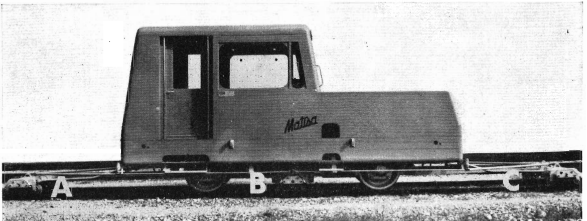
The Matisa track recorder. A, B and C are the small trolleys that, together with the driving wheels, register the track variations.
