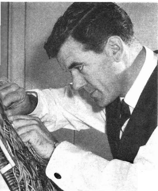
Mr. R. Simpson of the Computer Section wires a control panel for one of the new machines.
