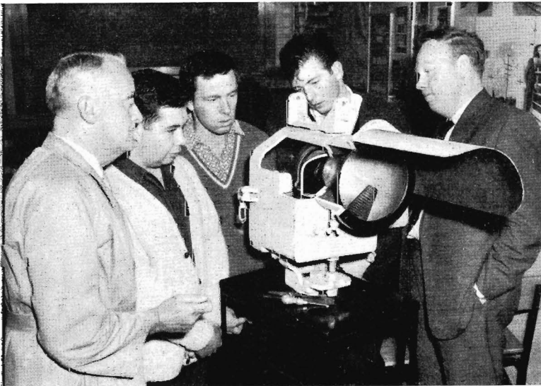
Instruction is being given on a searchlight signal. Cover is cut away to reveal electrical mechanism and optical equipment.
