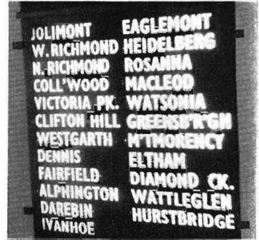
A slide has been projected on the glass screen of the prototype indicator developed by Electrical Engineering Branch engineers. The actual screen is much lighter in tone; it has been darkened to facilitate legible reproduction.
