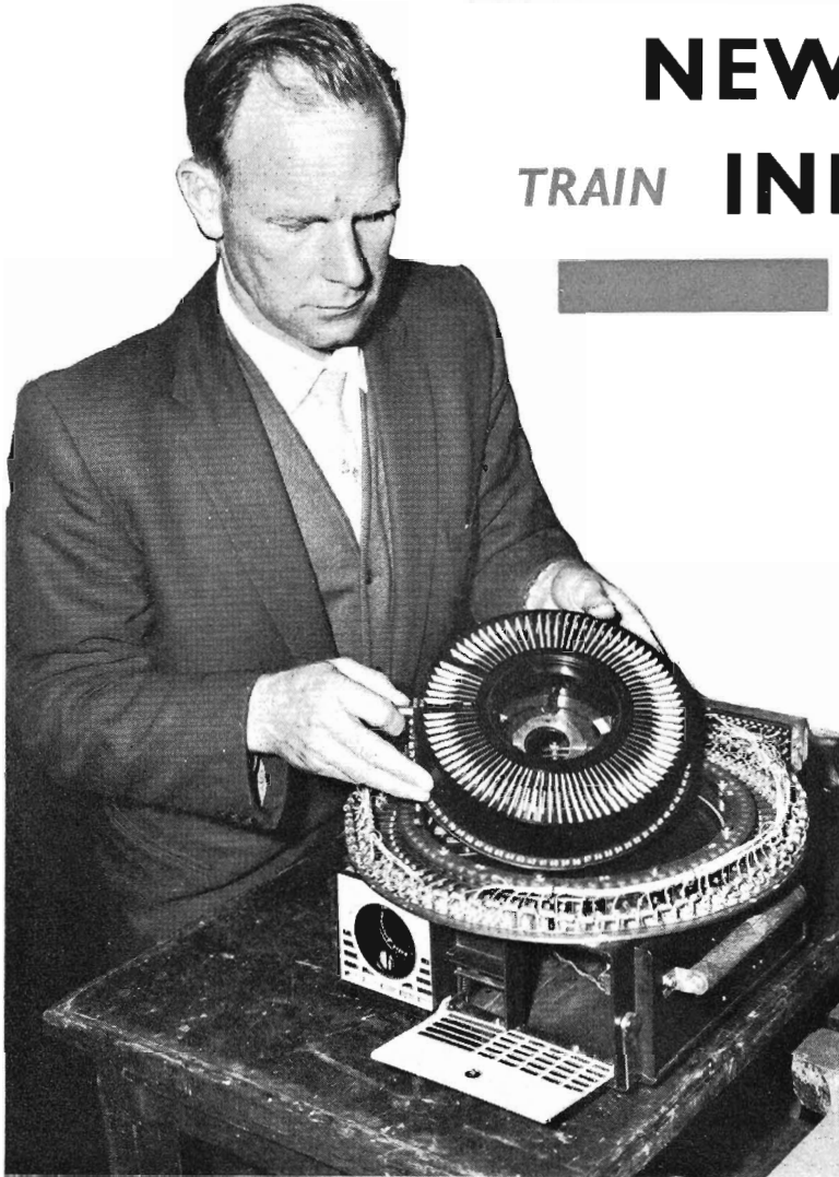
At the Testing Section, Mr. A. Firth, Engineer-in-Charge of Tests (Electrical), is placing a magazine of slides in the Carousel projector. On top of the projector is the mechanism that selects the slide to be projected.
