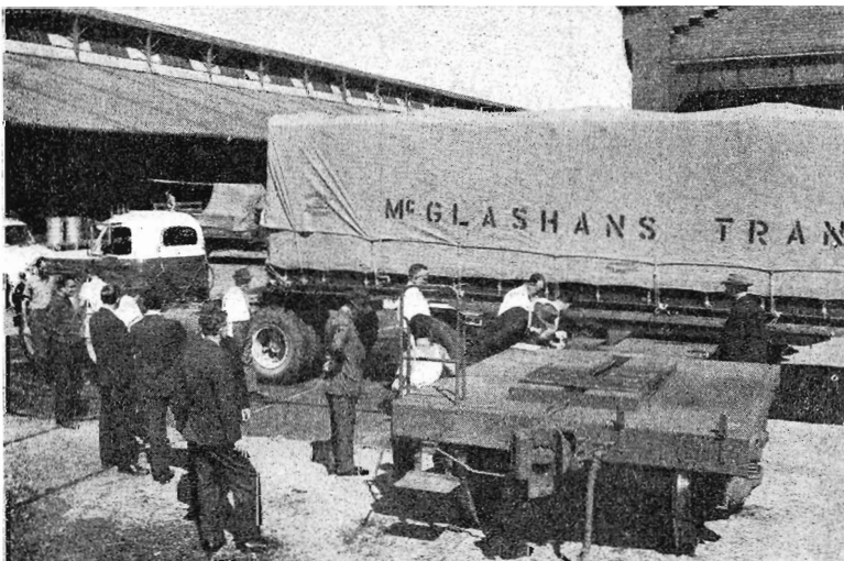
The first consignment sent by the new Flexi-Van service to Mildura, is shown being loaded on to rail wagon at Melbourne Goods.
