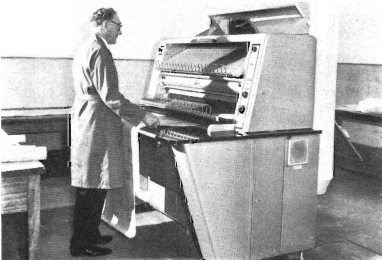
Leading Plan Printer E. Sullivan puts a tracing through the one-step ammonia printing machine.
