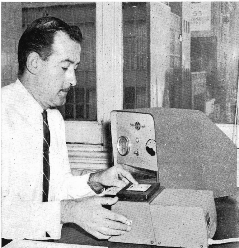
The new country periodical plastic tickets that were introduced last month ( News Letter , page 56) are prepared by sandwiching the paper ticket between two sheets of transparent plastic which are then sealed by pressure and heat in the larger of the two machines shown above. At the Ticket Supply Sub-division, Mr. M. Stone is completing a sealed ticket by trimming it in the smaller machine.
