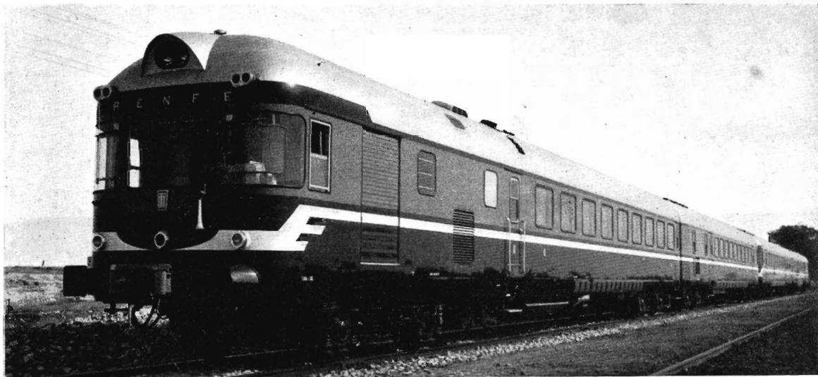
One of the new fast railcar trains which have been recently introduced on the Spanish National Railways is shown above. They have been named Tar Trains (Trenes Automotores Rápidos) and each unit consists of four coaches. Train sets can be made of up to 12 coaches, with multiple-unit control. Two diesel engines, with a combined rating of 1,700 h.p. are used for each set of four coaches. Transmission is hydraulic, by means of torque convertor. Coaches are air-conditioned and a kitchen-bar is installed.
