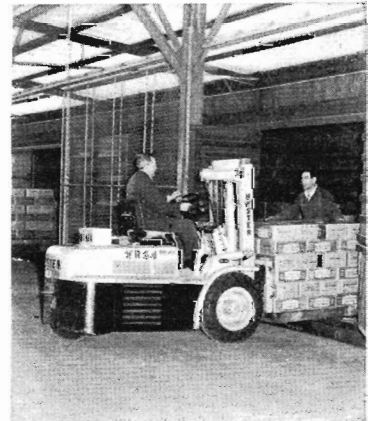
At the Melbourne Goods grain shed, medium sized fork lift trucks are ideal for handling dried fruit packages.
