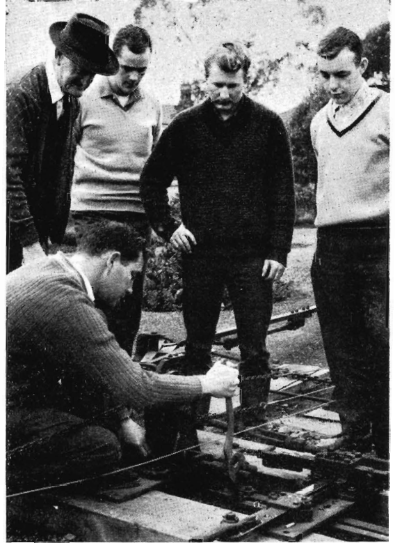
At the Mechanical Signalling School, Newport, the instructor explains the adjustment of a mechanical point detector.
